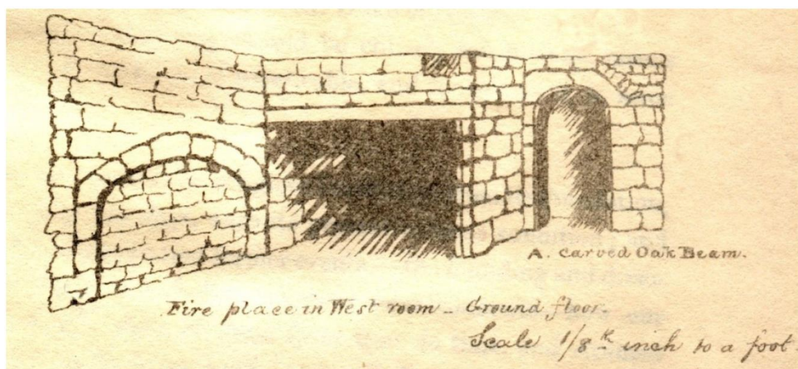
Figure 10: Sketch of West internal fireplace and removed cross wall with blocked arch, St Mary's Chantry (in Dickson 1852)
